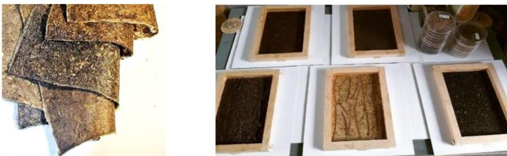
Image 8: Vinyl of gelatin and starch bioplastic with fibre. The optimal formula for the matrix was 10:3/4:2:1, which entails 100 g water, 7.5 g of gelatin, 20 g of glycerin and 10 g of vinegar for the mould used. The optimal amount of fibre added was 3 g dried or 20 g wet. It solidifies in 15 minutes, but to be completely dry takes approximately 96 hours.
