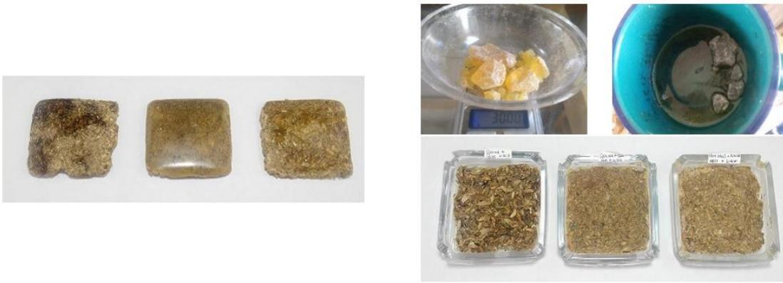
*Image 9: Bioplastic of pine resin. This material consists of three components: pine resin, beeswax and fibre. The wax is added to give fluency to the mixture. The optimal amount was 15 g resin, 15 g wax and 3 g dried fibre. The matrix is heated until it melts and then is cast in a mould with the fibre already inside it, stirred for a few seconds and left to dry.*
