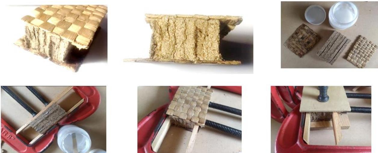
*Image 11: Bio-panel. A combination of the last two materials: agglomerate + bio-laminated weave. The agglomerate is glued by the faces with starch bioplastic and subjected to pressure. Then, two pieces of laminate are set under and over the agglomerates and glued with starch bioplastic applying pressure too. The result is a light and hard piece of a sandwich of water hyacinth that supports large amounts of weight.*
