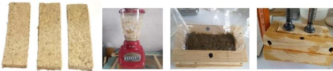
Image 6: Agglomerate. Material made of 100% fibre, previously treated with water immersion of 7 days, only subjected to pressure in a mould to take form and expel most of the water. This presentation of bars was weak in its face, but very strong when it was resting on its edges.
